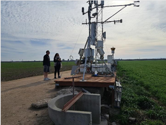
Figure 2 Aaron and Rachael check out a heavily instrumented eddy covariance tower on a Californian dairy farm
