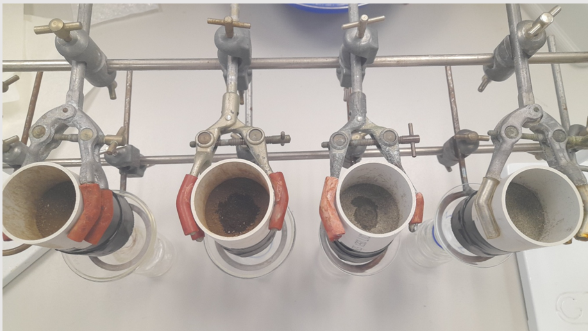
Mini leaching column experiments investigating vertical transport of Toxoplasma gondii oocysts through soils.
