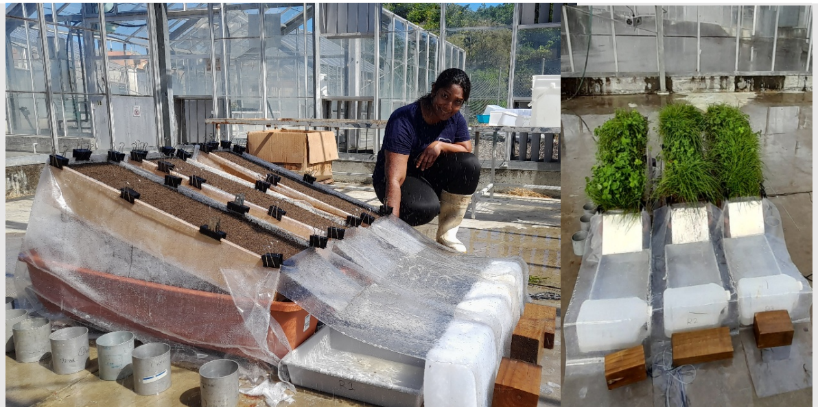
Rainfall simulation experiments investigating the transport of Toxoplasma gondii oocysts under bare and pasture-covered soil systems.
