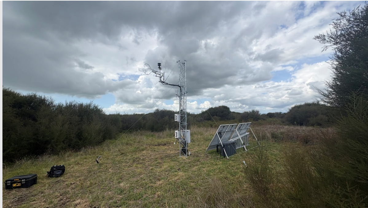
Figure 1. Eddy covariance tower installed in a retired paddock on drained peat that is now supporting a mix of weeds and manuka.
