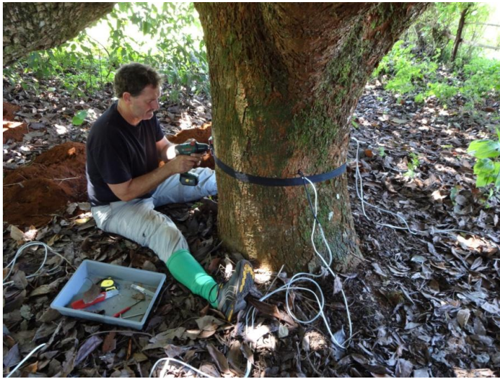
Steve installing heat-pulse sap flow probes to measure avocado tree water use.
