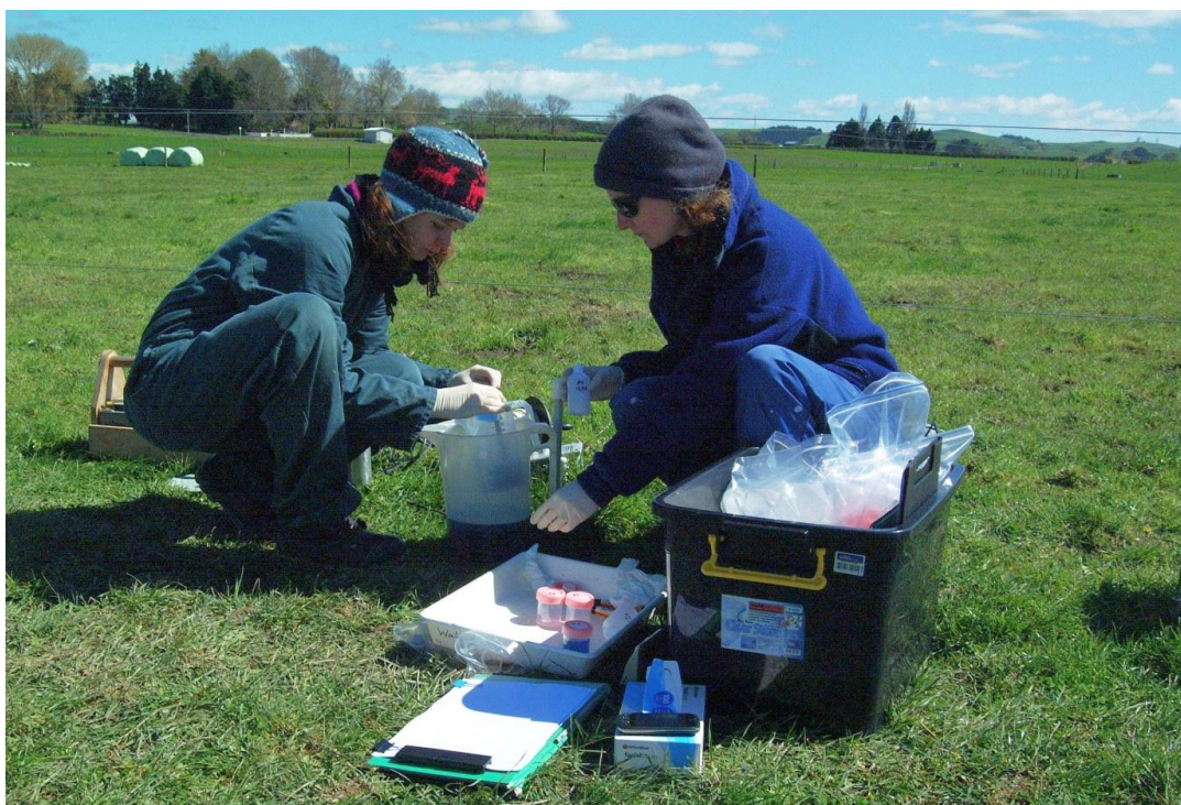
Fig. 1: Juliet Clague (right) and internship student Maike Rath (left) conducting a push-pull test to investigate groundwater denitrification in the Toenepi catchment.
