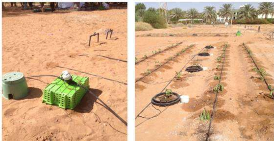
Left panel shows the flow meter (Sensus model) used to record irrigation volumes. This device produces one electronic pulse for every litre of water. Right panel shows the eggplant crop a few weeks after planting. Irrigation is regulated using a pressure-compensated dripper (4 L/h) for each plant. The black pots on the right panel are the four lysimeters that are buried below the soil, to a depth of about 70 cm.
