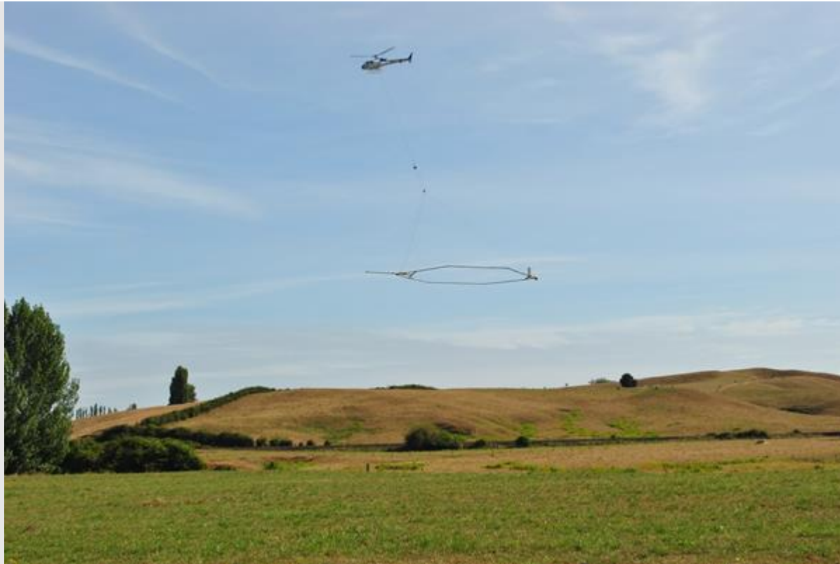
Fig. 2: SkyTEM survey being conducted in the Piako River headwater catchment in February 2019 (Photo: Aldrin Rivas).
