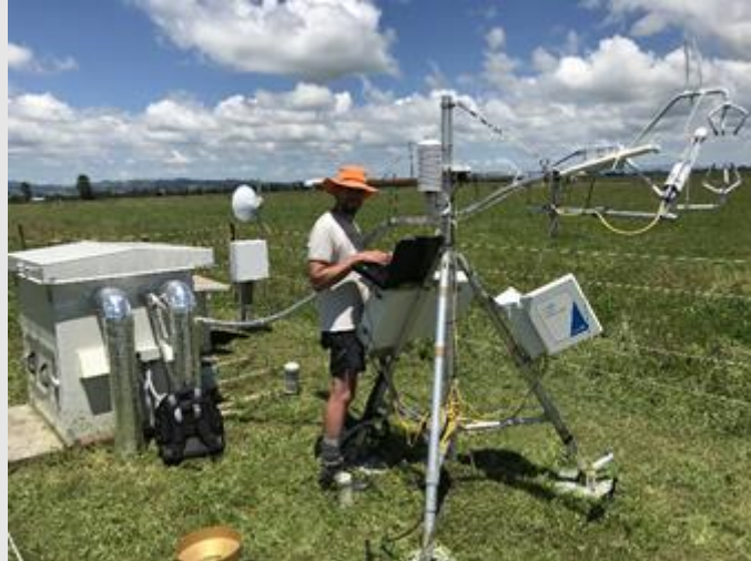
Figure 12: Chris Morcom at the Gamma Farm EC site. Instruments on the right measure \text{CO}_2 and \text{H}_2\text{O} fluxes, with a sample tube delivering air to the quantum cascade laser housed in the large temperature-controlled box, left.
