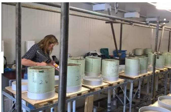
Trish Fraser seals a lysimeter onto its base
