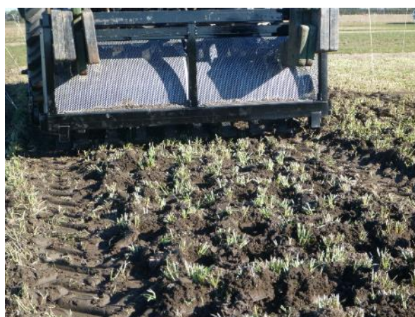
Compaction simulation from the Hoofiroller
