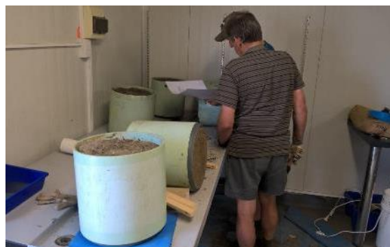
Richard Gillespie and Michelle Peterson weigh the bases containing saturated sand prior to lysimeter installation
