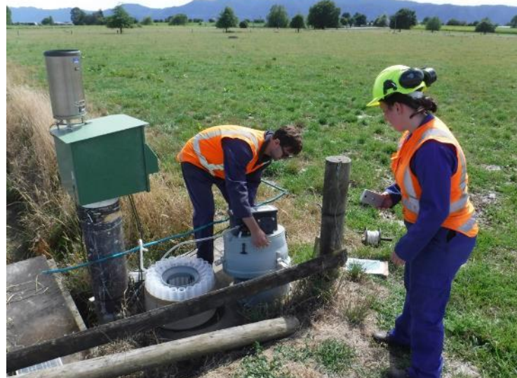
Fig. 3: Tasman McKelvey explaining our set-up for flow-proportional sampling of drainage water to Kathryn Gale from Kāi Tahu ki Otago.
