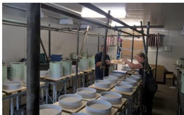
Frank Tabley and Will Burrows prepare the lysimeter contact area ready for positioning onto their bases
