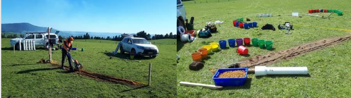
Photos: installation of fluxmeters in a field to be sown to hemp.
