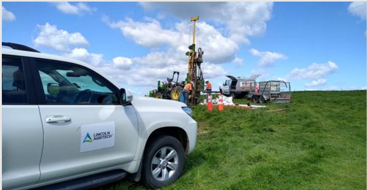
Figure 3: A 50 m deep borehole was drilled to gather detailed lithological information at 2 locations in each study catchment to cross reference with the geophysical data collected.
