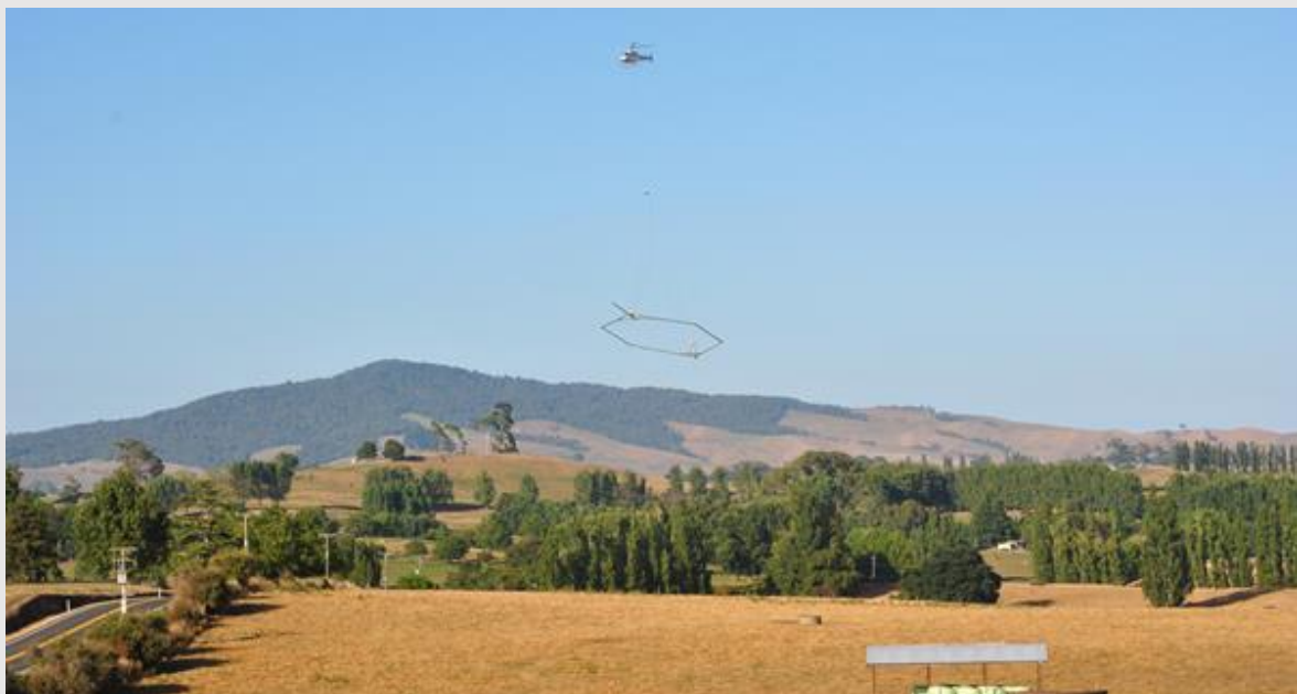
Figure 1: SkyTEM aerial survey carried out in the Upper Piako catchment in February 2019.
