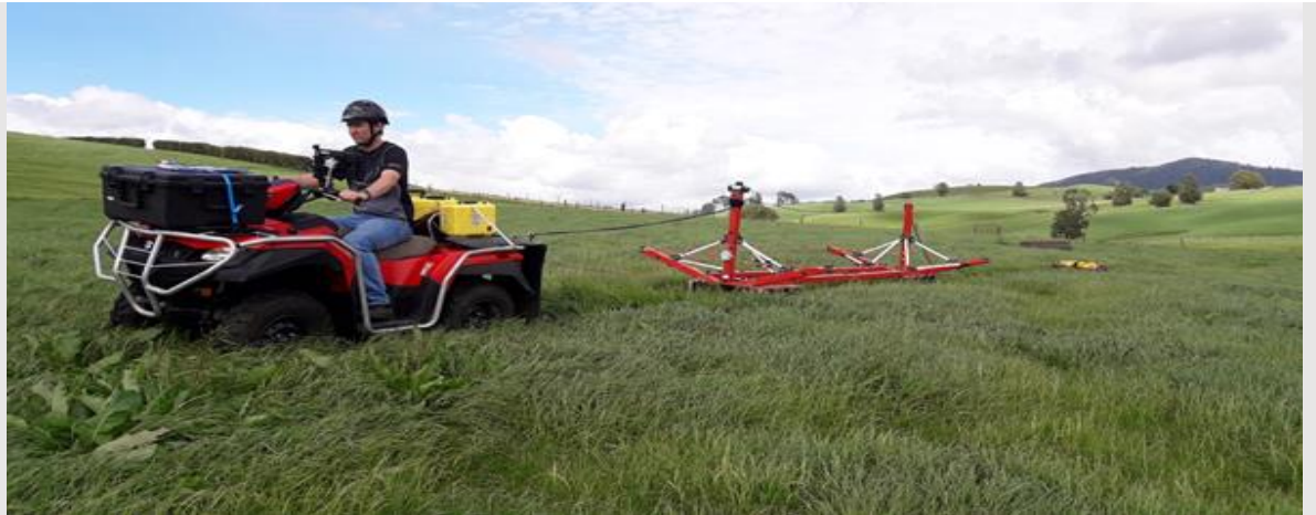
Figure 2: tTEM ground-based survey carried out in the Upper Piako catchment in November 2020.
