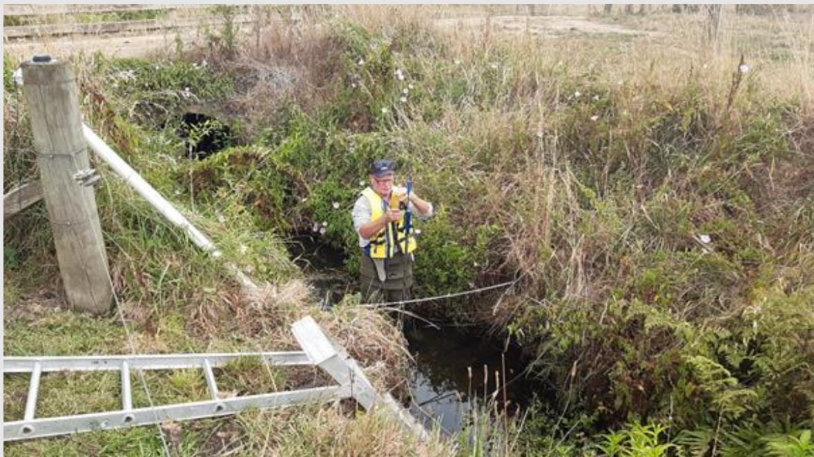
Figure 1: Stream gauging in the Upper Piako catchment to correlate flow and water level heights measured by the pressure sensor (in the PVC tube).
