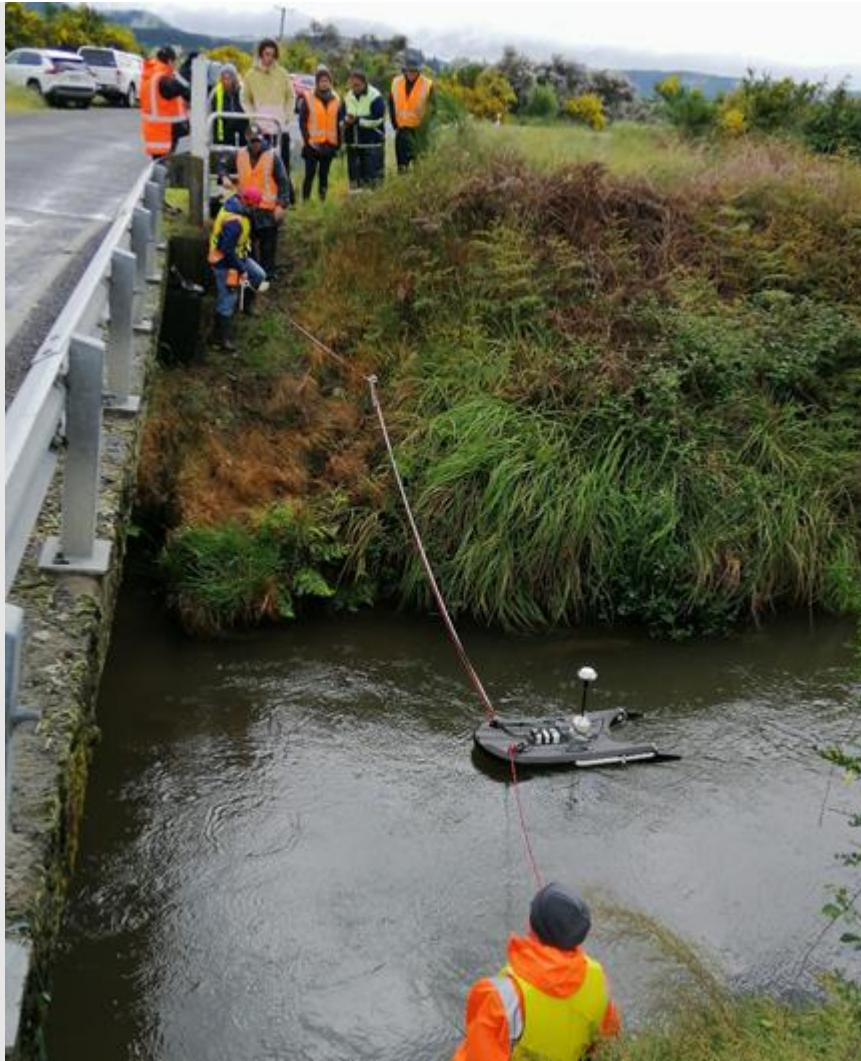
Figure 3: Stream gauging in the Waioatapu catchment using a RiverSurveyor.
