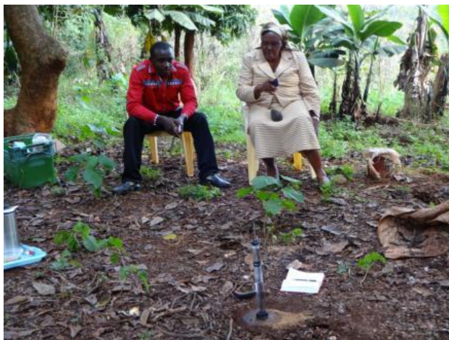
Michael Gitahi from Olivado (Kenya) explains the soil physics' details of a mini-disc permeameter (foreground) to Jacinta, an avocado farmer at Mangu near Thika.
