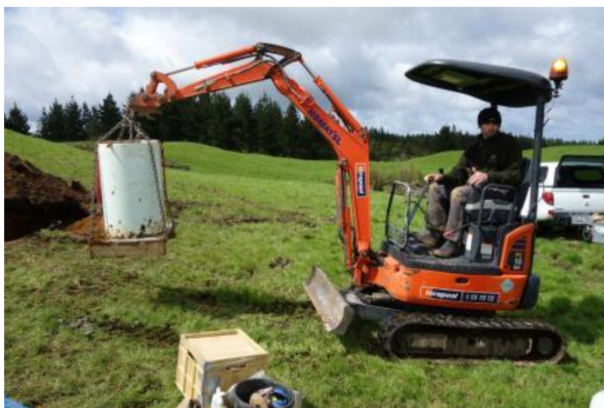
Photo 2: A completed lysimeter on the way to the trailer, during a fine spell, for transport back to Hamilton. Photo: Malcolm McLeod.
