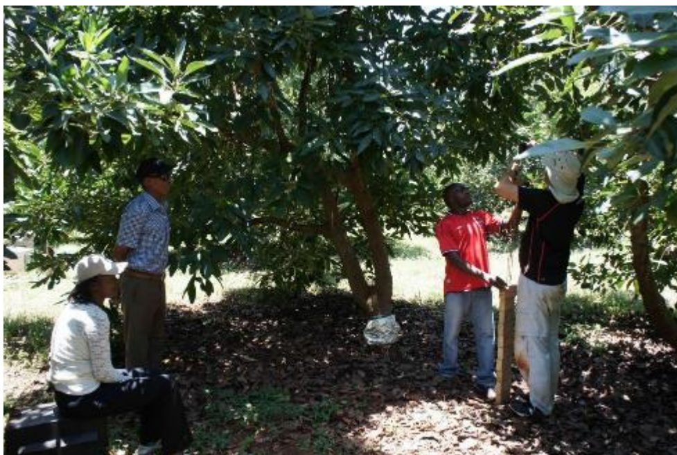
Steve Green (right) and Michael Gitahi from Olivado (second from right) installing 2 m long TDR rods on the farm of Mr Thomas Njui (second from left) under the watchful gaze of Sarah Murigi from Olivado (left). The tree in the middle is instrumented with our heat-pulse sap flow gear.
