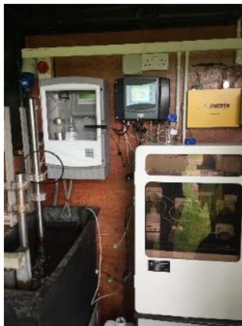
Right: Nitratax and Phosphax sensor used for high frequency nitrate and phosphate monitoring of water quality as part of the Agricultural Catchments Program in Ireland
