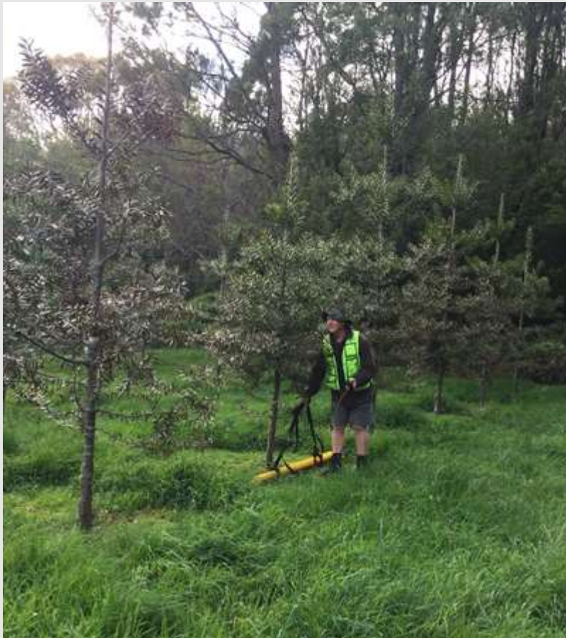
Using the DUALEM to characterise soil properties under a native forest planting
