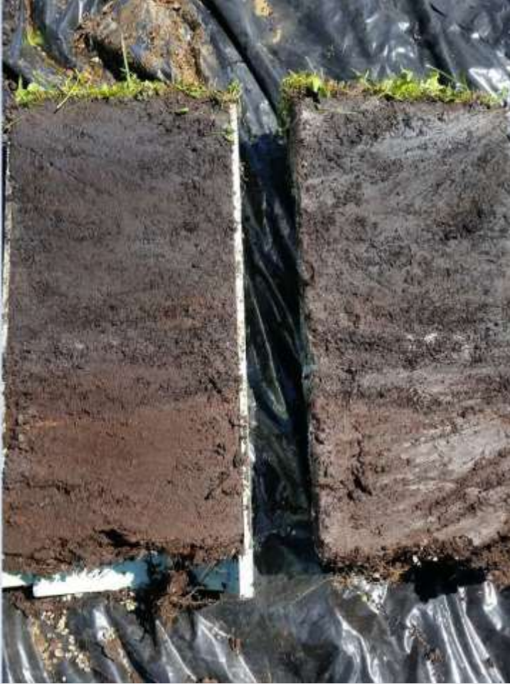
Photo 2. A destructed lysimeter containing a high risk peat soil for FDE management (Rukuhia peat)
